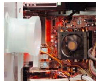
This heatsink funnel channels air directly outside the case
